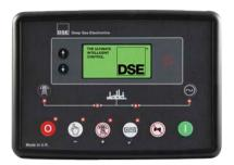
• Auto Module Control Panel, usually adopt control module of UK Deepsea DSE 6020 or Equal, is the configuration for nobody on duty generators control, This kind of panel adopts auto module control system, with large LCD display to show the menu.
